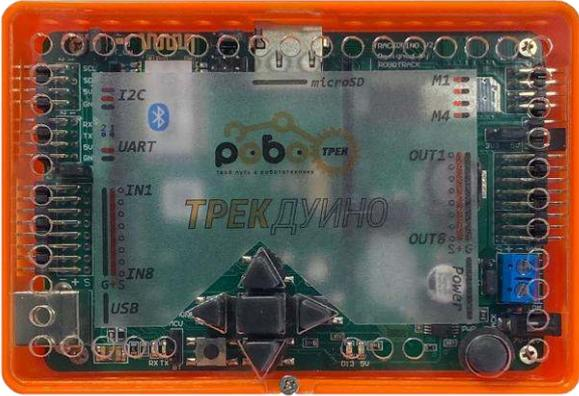
A green printed circuit board (PCB) for a controller, housed in a clear orange plastic enclosure. The board is populated with various electronic components, including a microcontroller, a USB port, a microSD card slot, and several pin headers. Labels on the board include "I2C", "UART", "microSD", "M1", "M4", "OUT1", "OUT2", "IN1", "IN2", "IN3", "IN4", "IN5", "IN6", "IN7", "IN8", "USB", "POWER", and "TREKDUINO". The board is connected to a blue USB cable. | <p>1</p> |
